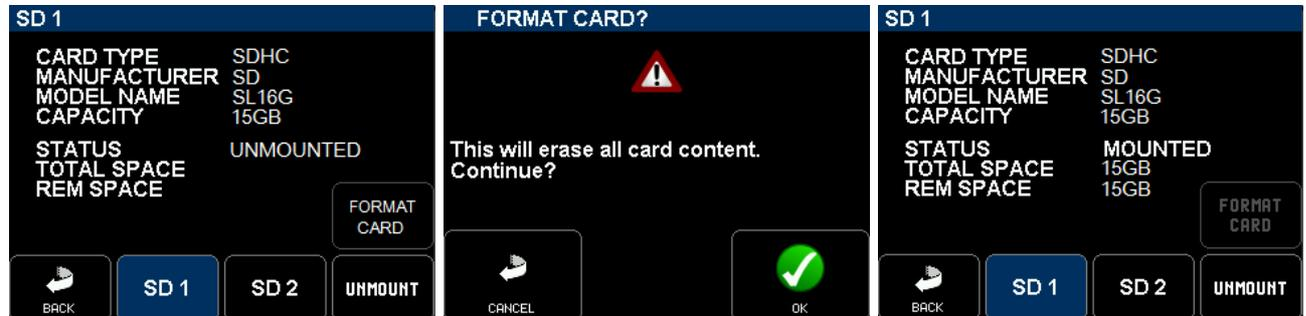
Insert a SD card in a slot, then press the Format Card
