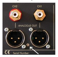
White arrow points to the rotary switch for the basic output level selection.
