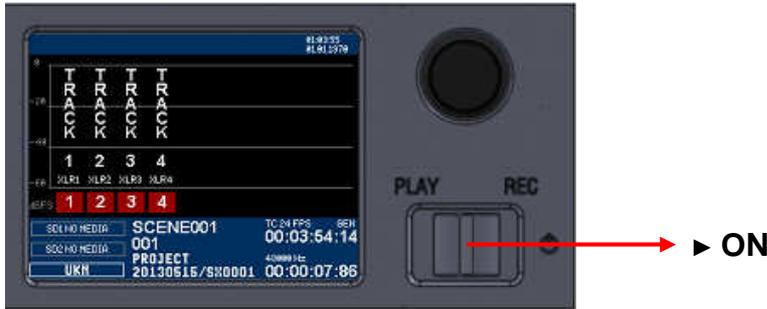
Press the toggle switch to the right to power on the SX-R4+ . A boot up screen is displayed for a couple of seconds, followed by:
