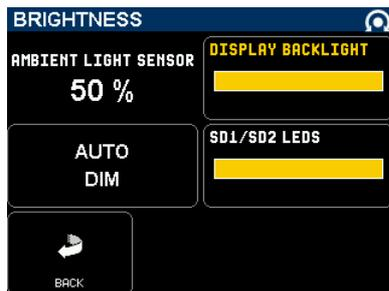
[LIGHT SENSOR] indicates the ambient light intensity
