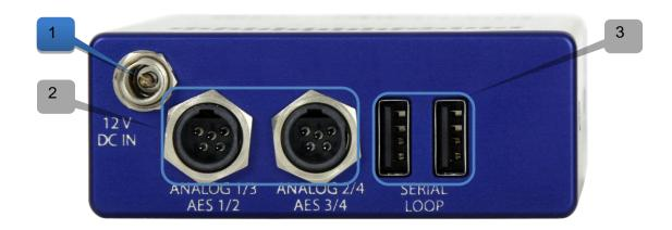
1. DC Power Input - The QRX uses a Switchcraft 761K connector.
